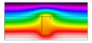
• Exterior Walls: Typically ranging from 0.15 to 0.35 W/m<sup>2</sup>·°C, U-values for light steel framing exterior walls are
