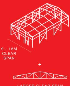
LARGER CLEAR SPAN WITH THE USE OF TRUSSES
