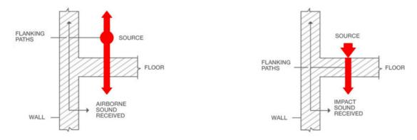
The acoustic performance of LSF systems can vary depending on specific design details, construction techniques, and the choice of materials. Acoustic performance is typically quantified using standardised metrics such as Sound Transmission Class (STC) and Impact Insulation Class (IIC) ratings. These ratings indicate the ability of a construction assembly to reduce airborne and impact noise transmission, respectively.
